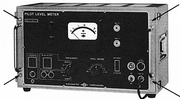
Fig. F1. How to Dismount the Pilot Level Meter, type BFM330
